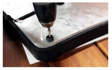
4. Attach the feet using the supplied longer screws.
