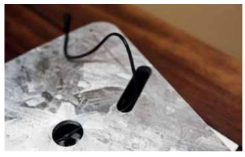
3. Put the extra weight on the bottom of the base making sure the holes match up. Push the two cables through the two outer holes.
