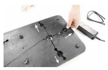
2. Push all the cables deep into the recesses. Choose each time the recess nearest to the next base (this only applies to the 60x30 and 30x30 cm bases).
